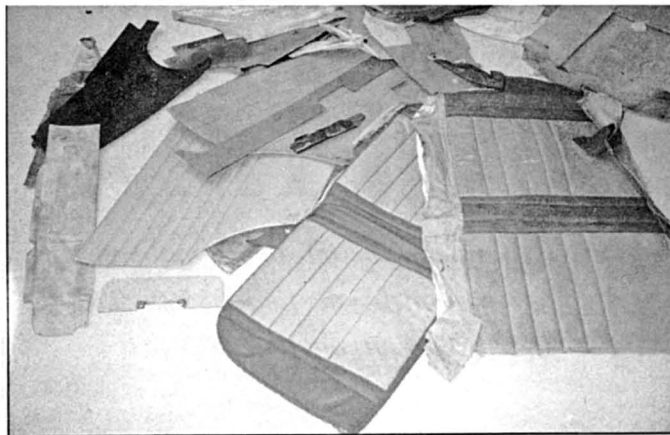
Part of the stock of original Mini-trim parts that Newton Commercial assembled as patterns to copy before they went into full-scale production
